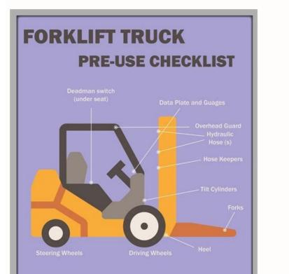
An operator should inspect the forklift truck every day, including at the beginning of each shift, and before using each time.
